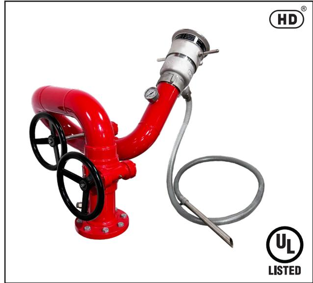
The Monitor has welded Stainless Steel 4 inch (100mm) waterway. Vertical and horizontal rotation is through stainless steel swivel joints with double row of stainless steel ball bearings. Both vertical and horizontal movements are controlled with handwheel driven enclosed worm gear.
