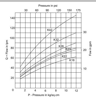
Q =K  $\checkmark$  P where P is supply pressure in kg/sq.cm, K=nozzle constant (K-factor) in metric. US K factor = Metric K factor ÷ 14.2745 K-Factor Tolerance = 2.8 K (Metric)
